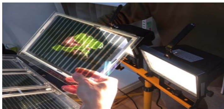
Figure: Large-area organic PV module with 9.5%.
